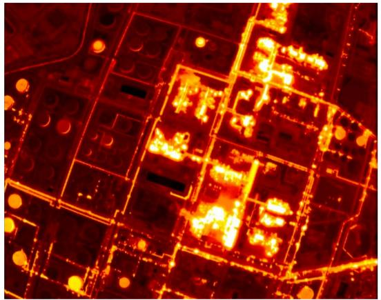
Stanlow, Liverpool. Night time imaging permits 24 hours energy use monitoring. Image taken from an aircraft with an engineering model of our space camera compared with typical visible photographs.
